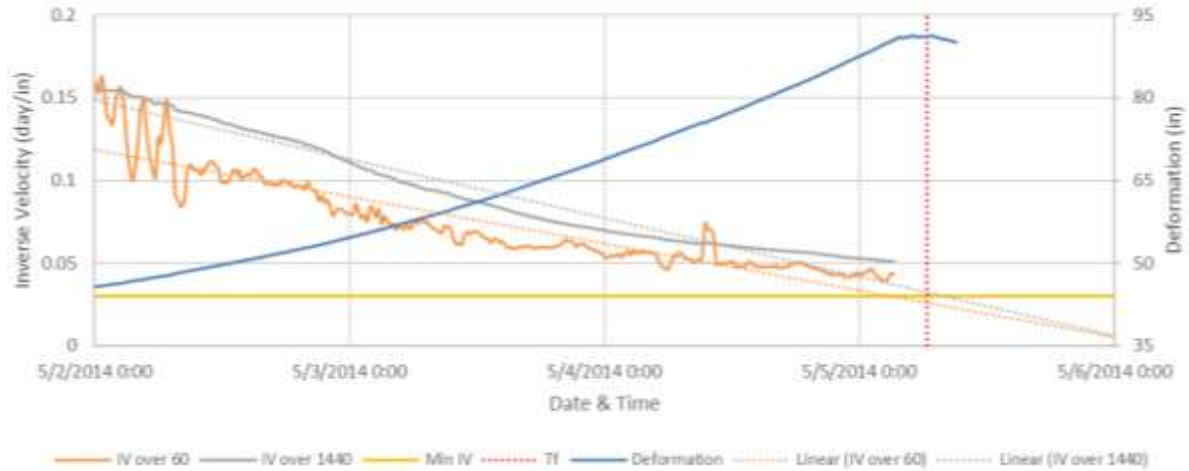
Figure 6. Demonstration of the use of minimum inverse velocity to analyze a failure 2 h before the failure at location X. The blue line represents deformation; orange line represents inverse-velocity averaged over 60 min, the gray line represents inverse-velocity averaged over 1440 min. Dotted orange and gray lines represent the extended best fit lines of the data to help predict the time of failure. The red dotted line represents actual time of failure. The yellow horizontal line represents the minimum inverse velocity.
