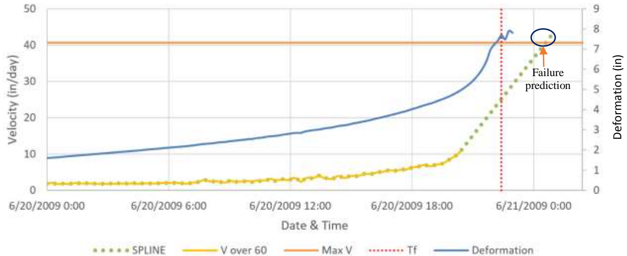
Figure 9. Demonstration of the use of maximum velocity for slope failure prediction at location B. The blue line represents deformation; yellow line represents velocity averaged over 60 minutes. The green dotted line represents the extended SPLINE to help predict the time of failure. The red dotted line represents actual time of failure. The orange horizontal line represents the maximum velocity.
